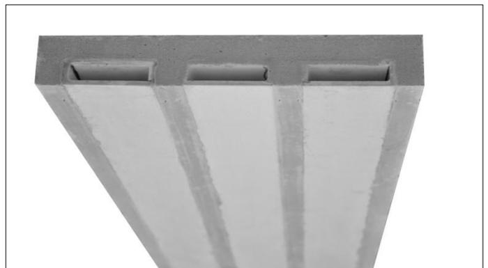
Figure 4. Light weight floor element made of UHPC and GFRP tube elements – student work by Magdalena Lang and Romana Streitwieser (TU Graz, 2011).
