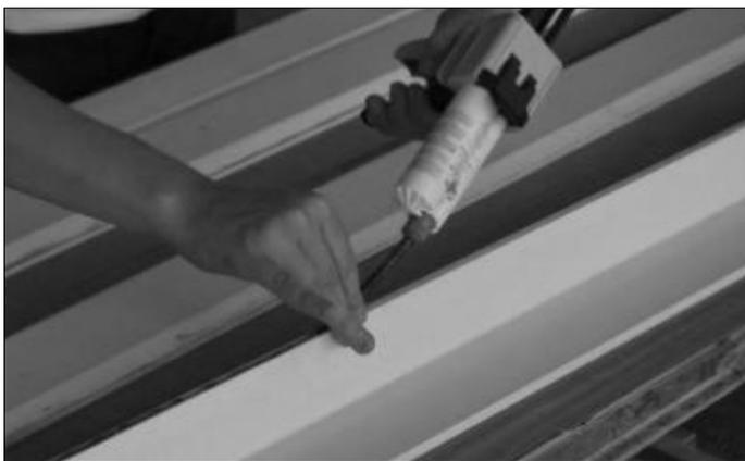
Figure 6. Fabrication of a GFRP tube profile by conglutination of two angles.
