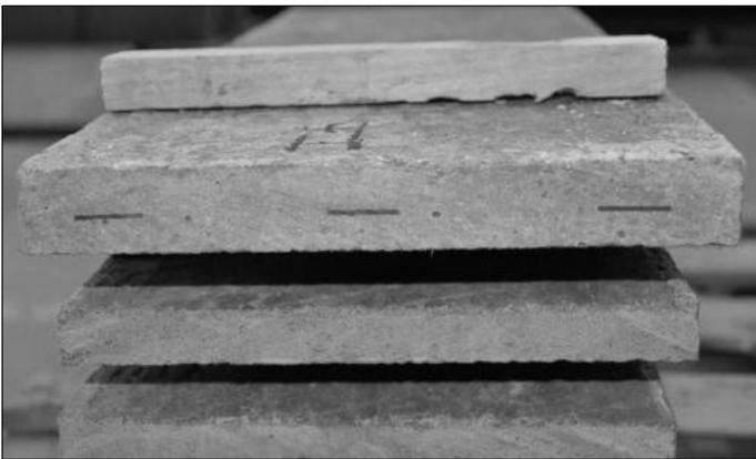
Figure 13. UHPC plates with and without centric CFRP lamellae (test series 1 and 2).
